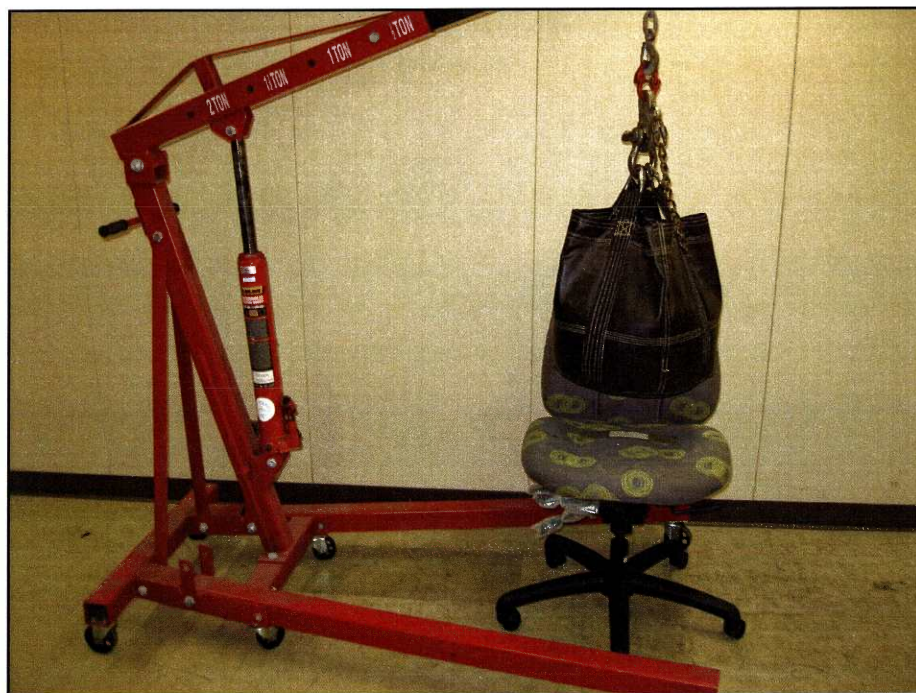
Figure 3 : Dynamic drop test set-up
