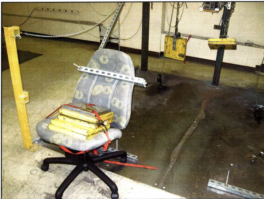
Figure 12 : Backrest durability test set-up (Type I)
