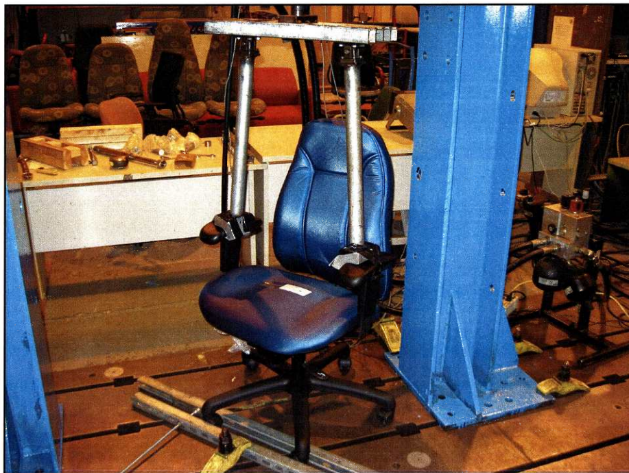
Figure 14 : Arm durability test set-up
