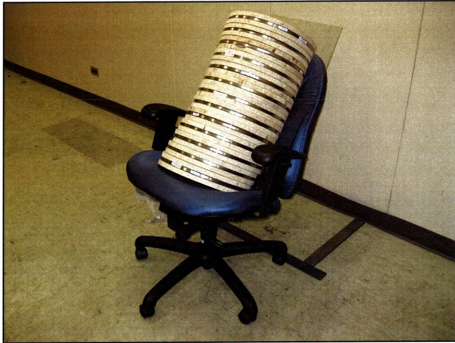
Figure 7 : Rear stability test set-up (Type I)
