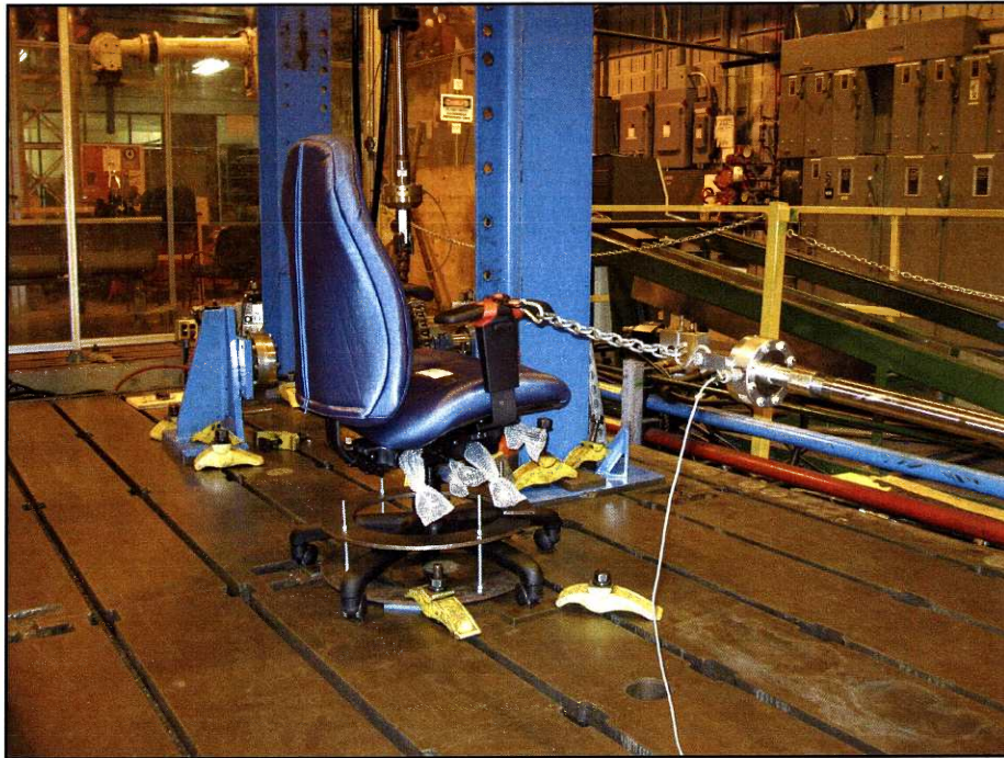
Figure 11 : Horizontal arm strength test set-up
