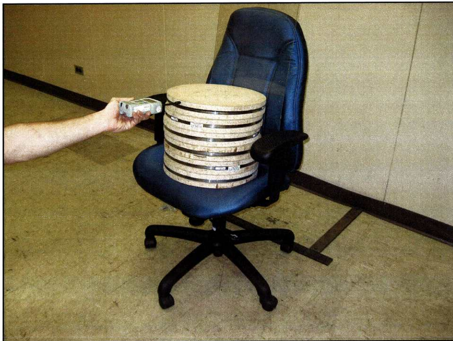
Figure 8 : Rear stability test set-up (Type III)
