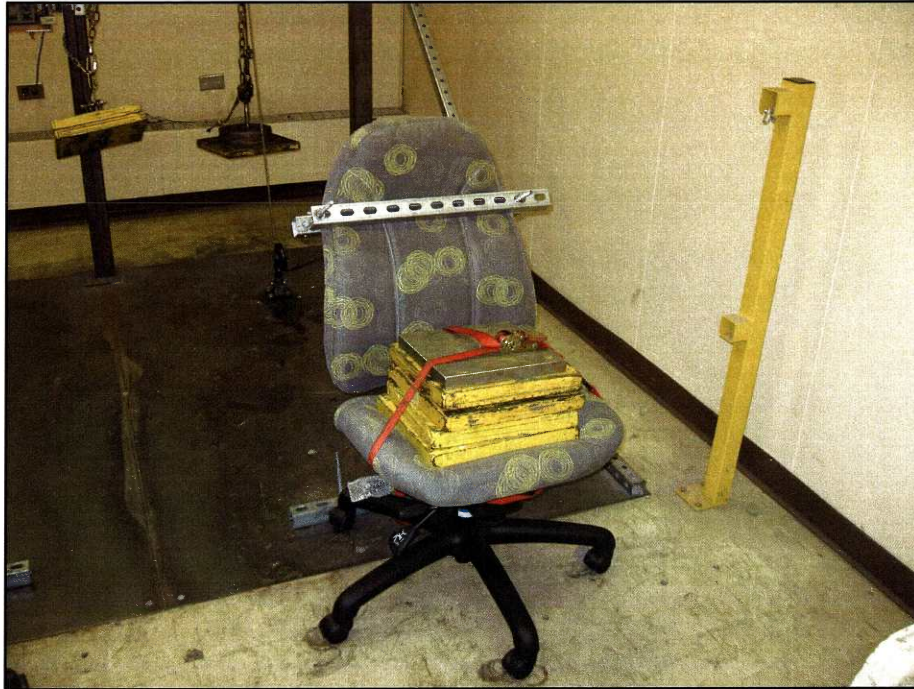
Figure 13 : Backrest durability test set-up (Type III)
